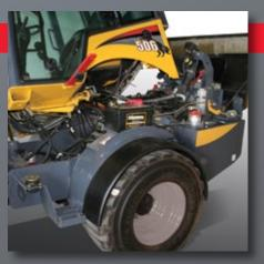
SERVICE ACCESS is made easy with a large engine hood that provides access to the engine, coolant and hydraulic oil. A tiltable, gas-spring assisted, isomounted operator platform lifts for easy maintenance access to the hydraulics and battery.
