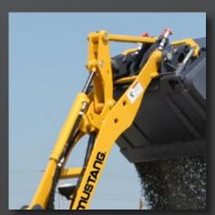
AN INTELLIGENT DESIGN A ensures that the hydraulic hose lines and loader linkage cleverly recess into the lift arm when raised to full height, protecting the hydraulic lines when lifting or dumping.
