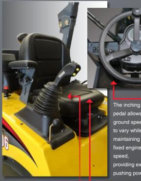
Multi-function joystick controls lift arm, bucket and float functions, as well as travel direction and auxiliary hydraulics. On models 306, 406 and 506, it controls twospeed and differential lock.
