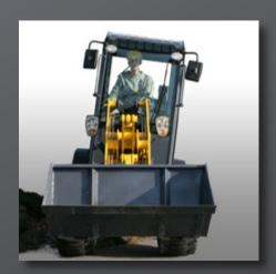
**STAY GROUNDED** with an oscillating chassis, 10 degrees in either direction, that maintains machine traction. Even on uneven terrain, the oscillation keeps the tires in contact with the ground.
