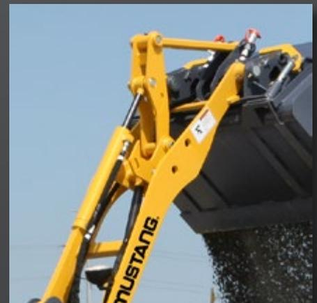
**AN INTELLIGENT DESIGN** ▲ ensures that the hydraulic hose lines and loader linkage cleverly recess into the lift arm when raised to full height, protecting the hydraulic lines when lifting or dumping.
