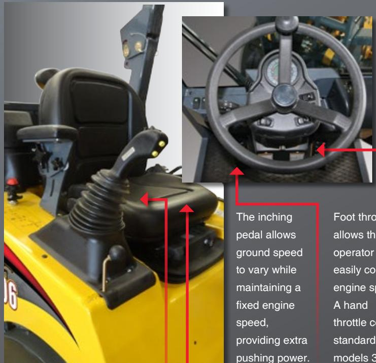
Multi-function joystick controls lift arm, bucket and float functions, as well as travel direction and auxiliary hydraulics. On models 306, 406 and 506, it controls two-speed and differential lock.
