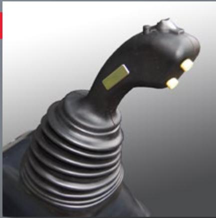
**MULTI-FUNCTION JOYSTICK** ▲ controls lift arm, bucket, and auxiliary hydraulic functions, as well as the float function. Travel direction, differential lock functions and two-speed are activated by switches and push buttons on the joystick.
