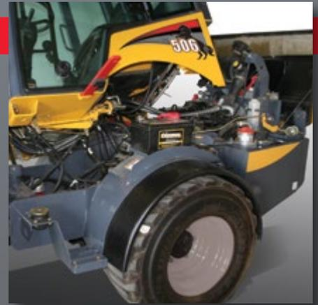
**SERVICE ACCESS** ▲ is made easy with a large engine hood that provides access to the engine, coolant and hydraulic oil. A tiltable, gas-spring assisted, iso-mounted operator platform lifts for easy maintenance access to the hydraulics and battery.
